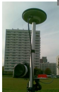
Figure 1. IMU and camera coordinate systems (Kolecki & Kuras, 2011), and the portable MMS prototype
